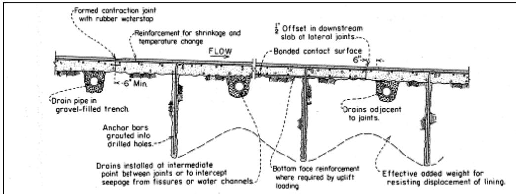
Figure 7 Typical Floor Lining on Rock Foundations
