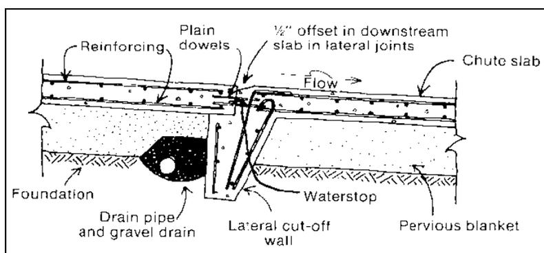
Figure 6 Typical Floor Lining on Earth (Soil) Foundations
